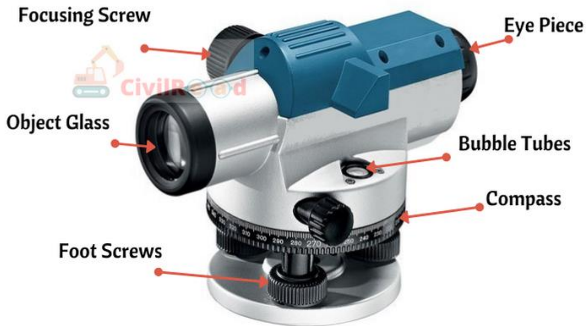
Components of Dumpy Level
